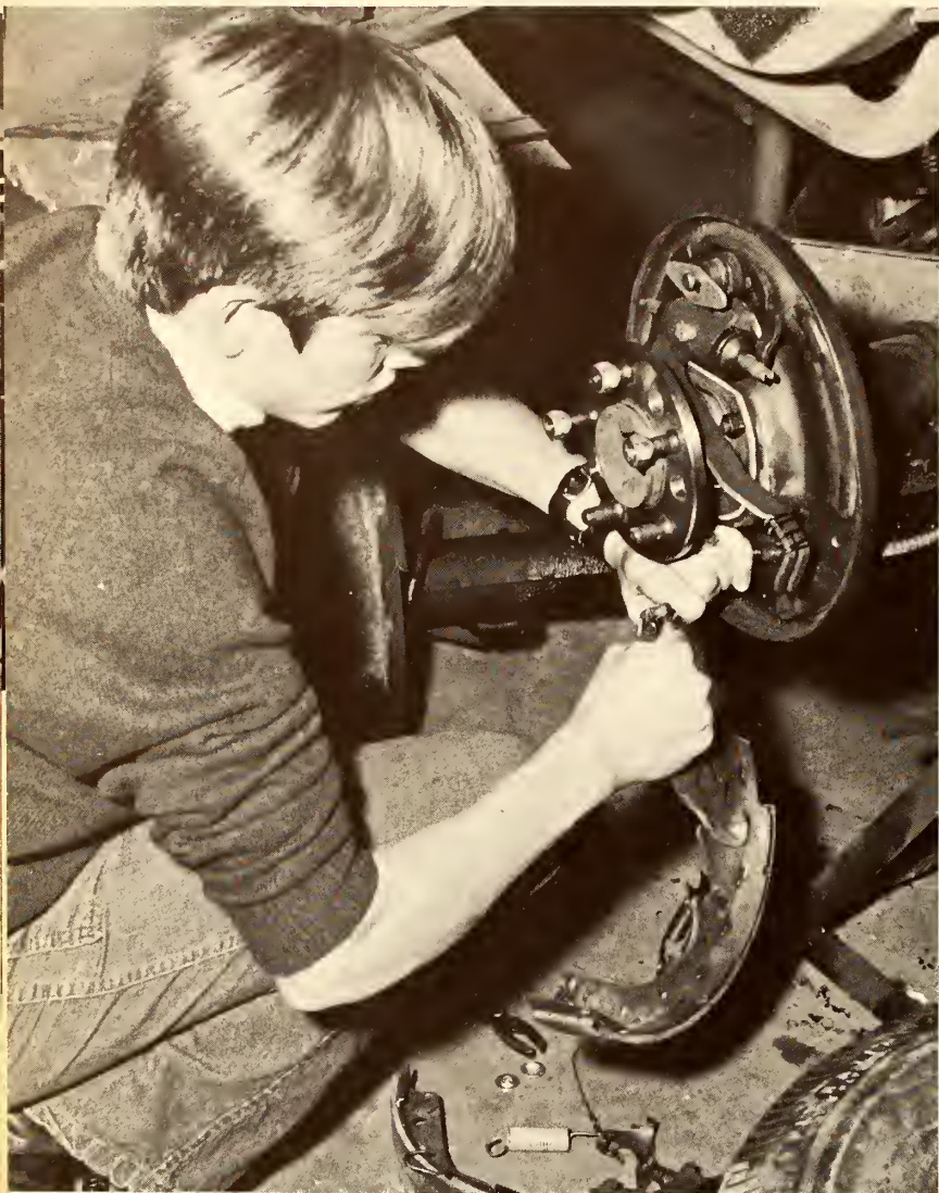
Students enrolled in auto mechanics class experience difficult tasks such as the changing of brake shoes of the braking system as this future mechanic is doing.
